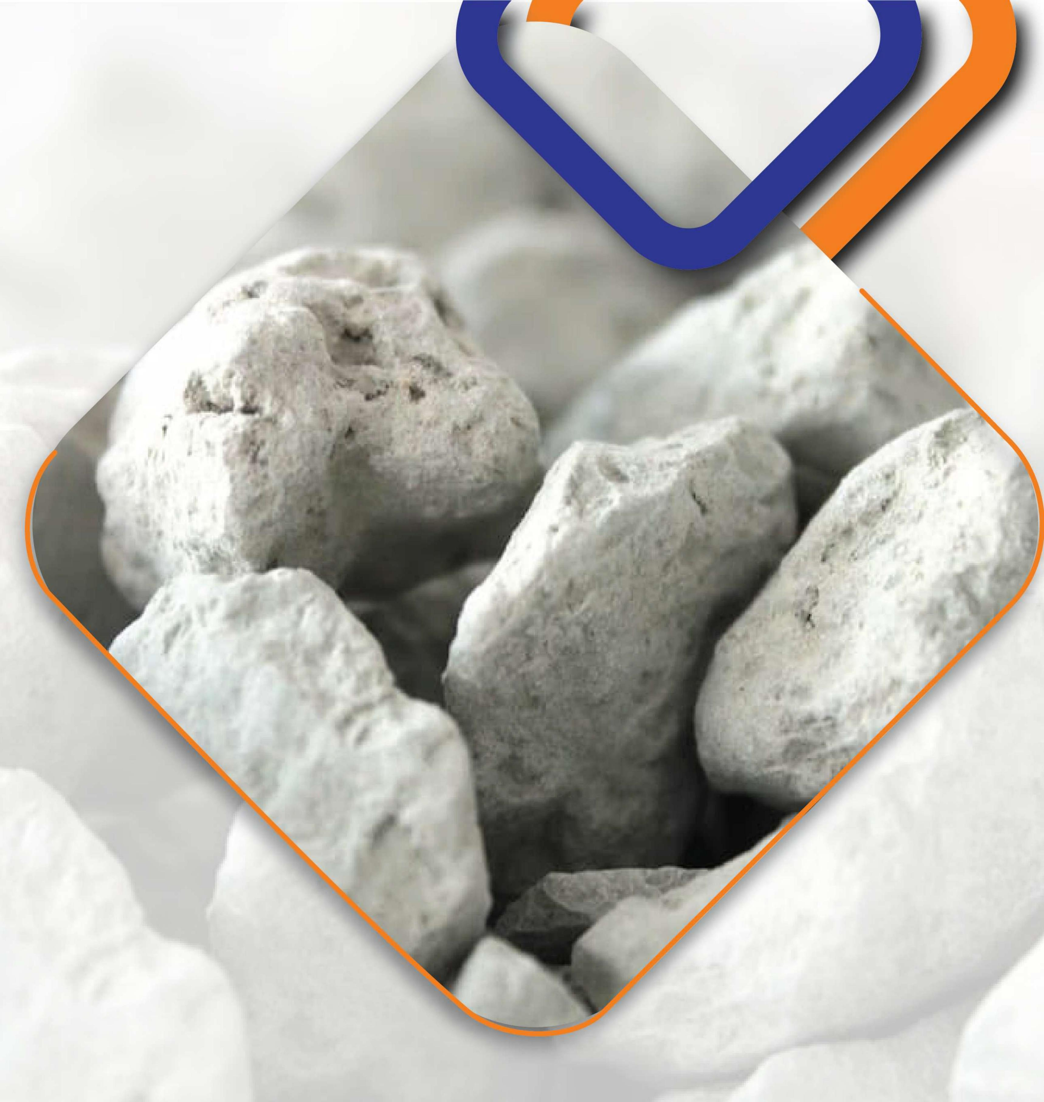
Moreover, Arzesh Afarin's bentonite products, with swelling indices between 15 and 30 and fluid loss below 16 ml, effectively perform sealing and protection of the wellbore.
